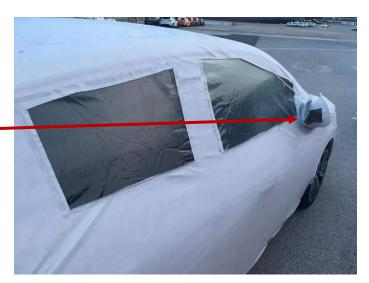
The wing mirrors should be usable, i.e. the FBC should fit correctly and have full transparency for the mirror (this picture is not a good example!)
