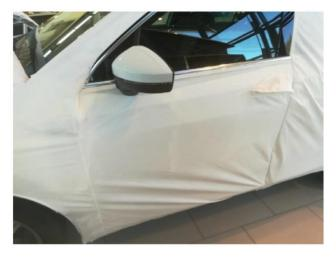
Good practice is to use "integrated doors" where the cover is secured with adhesive tapes around the driver's door so that the whole of the side window can be kept clear. This improves visibility considerably.
