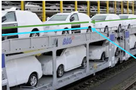
from a working height of 2 m a fall protection of 1 m is required
