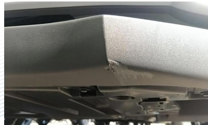
Scratches underneath the front bumper
