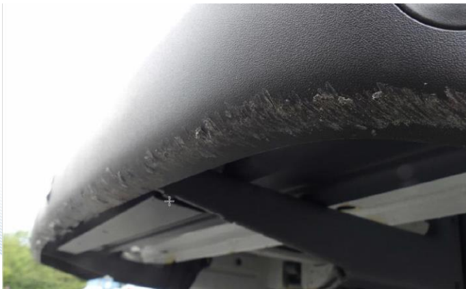
Scratches underneath the front bumper
