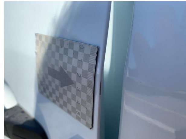
Panel-edge chip left front driver's door
