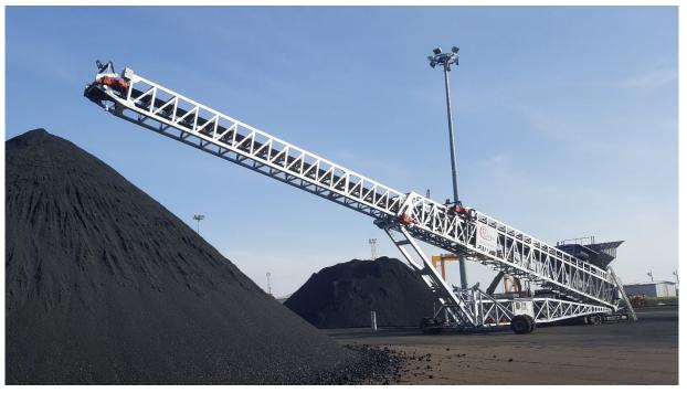
**Mobile belt conveyors** are one of the best material handling solutions for stacking any kind of bulk material when various materials has to be handled in various locations.
