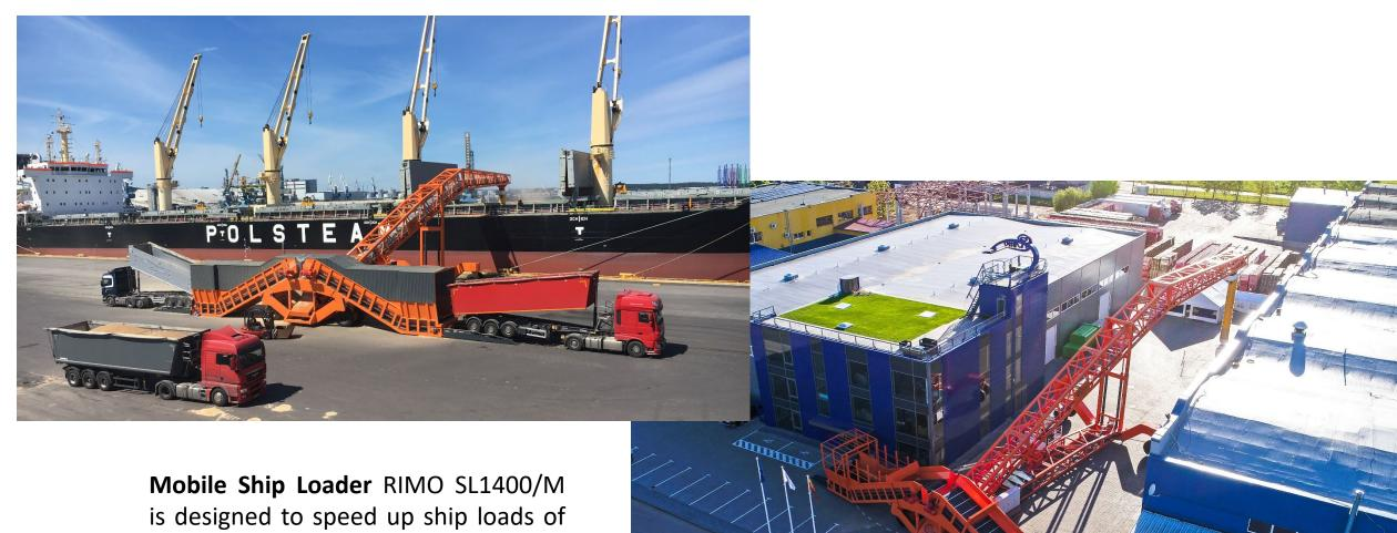
**Mobile Ship Loader** RIMO SL1400/M is designed to speed up ship loads of any bulk material – from aggregates to grains or wood pellets in ports.
